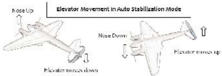
Figure 1 – 17 Elevator Auto Stabilization Mode
