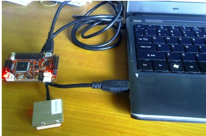
Figure 1 – 4 Connect APM Board and install driver
