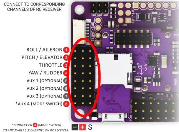
Figure 1 – 9 APM Board Input ports
