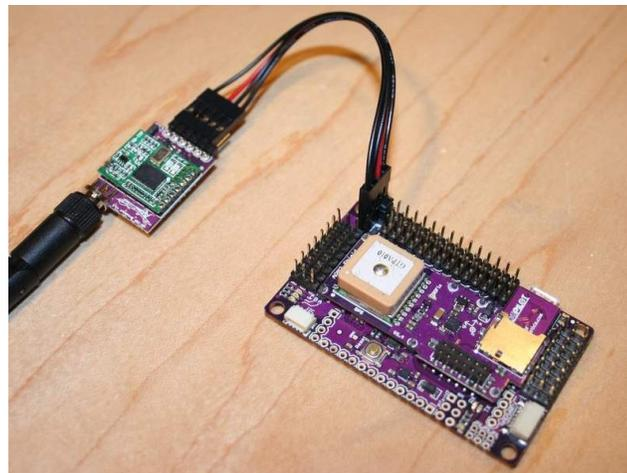
Figure 1 – 32 Connecting 3DR Radio Link
