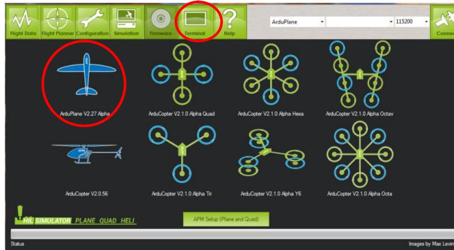
Figure 1 – 6 Upload Firmware
