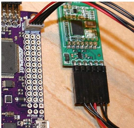
Figure 1 – 30 Connecting 3DR Radio Link
