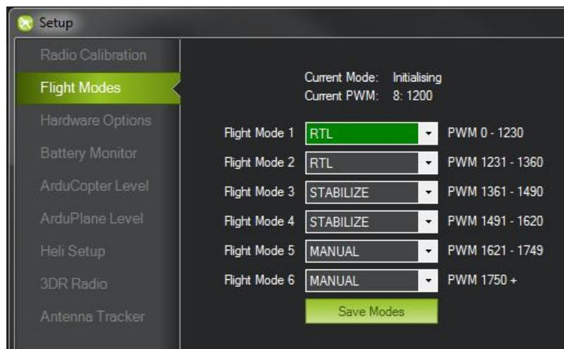
Figure 1 – 12 Setting Flight Mode on Mission Planner
