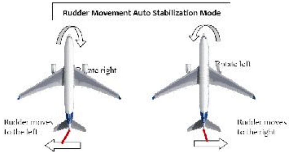
Figure 1 – 18 Rudder Auto Stabilization Mode
