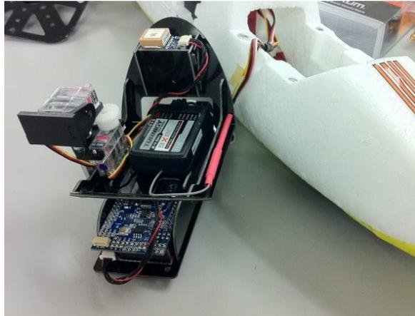
Figure 1 – 8 APM Board should securely installed and has no movement
