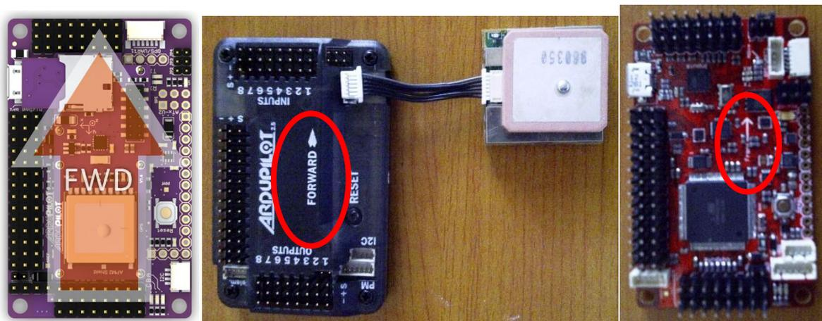
Figure 1 – 7 APM Board should be installed correctly
