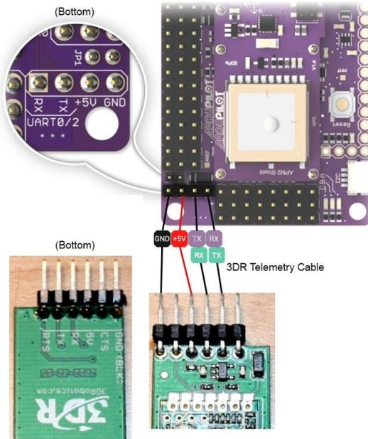
Figure 1 – 31 Connecting 3DR Radio Link
