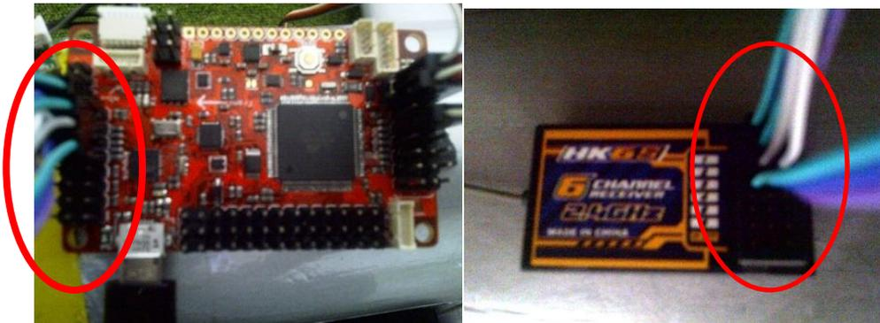
Figure 1 – 9 Connect APM Board Input ports to RC Receiver
